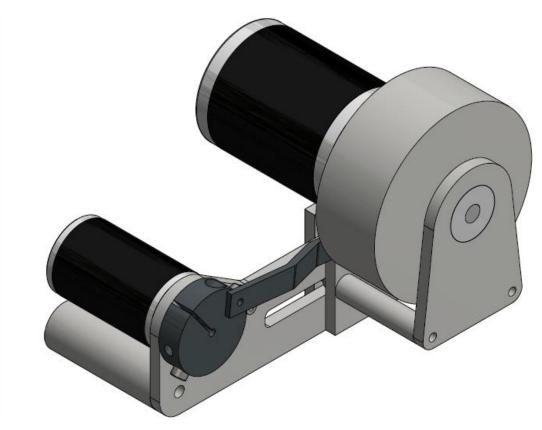
A four inch diameter\_wheel which actuates into the boulder.
